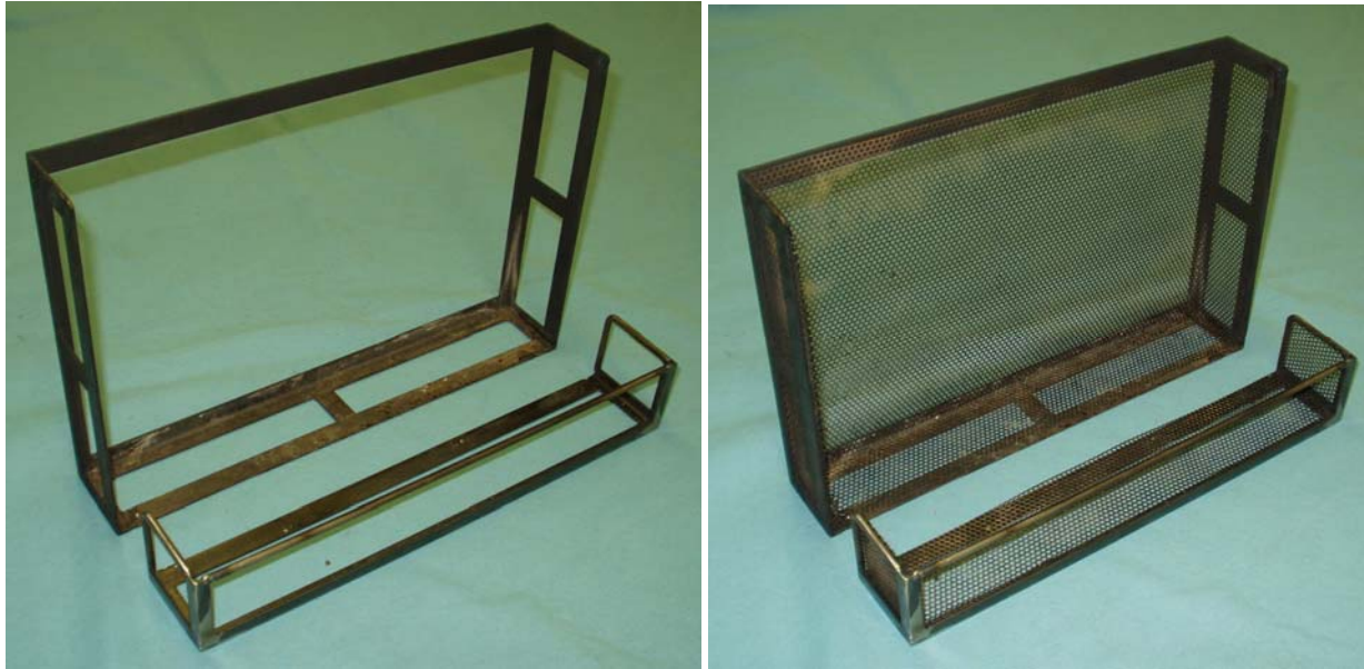
Photograph 1. The loose fill test inserts for small open flame testing. The photo on the right also includes screening material to help contain loose filling materials with small particles that may otherwise fall out of the small open flame mockup.
