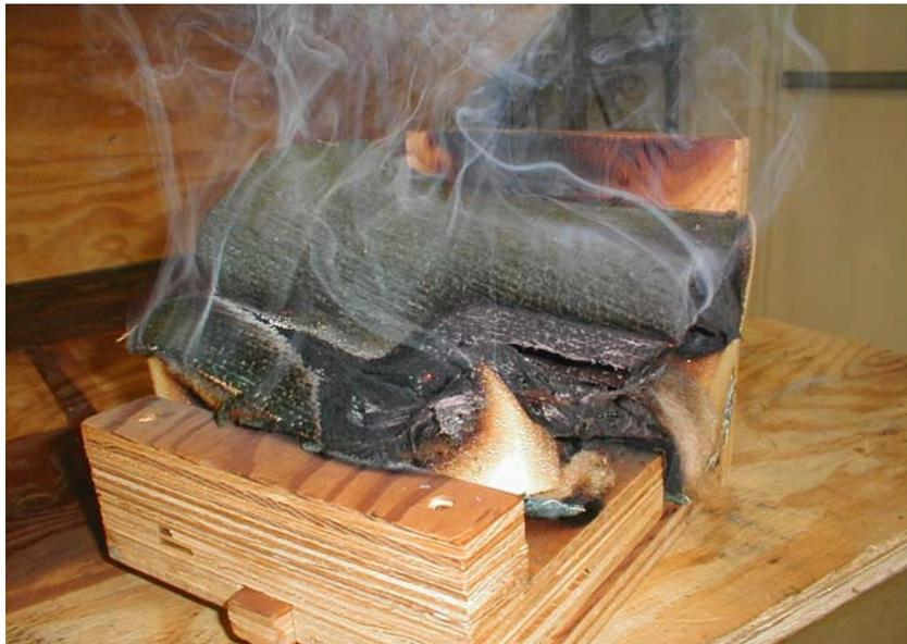
Figure 7. Post Test Mockup of Fabric 7 with UFAC Foam and UFAC Polyester Batting Still Smoldering
