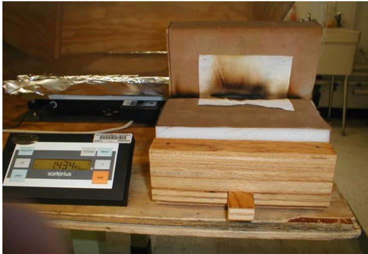
Figure 2. Post Test Mockup of Fabric 24 with Foam T
