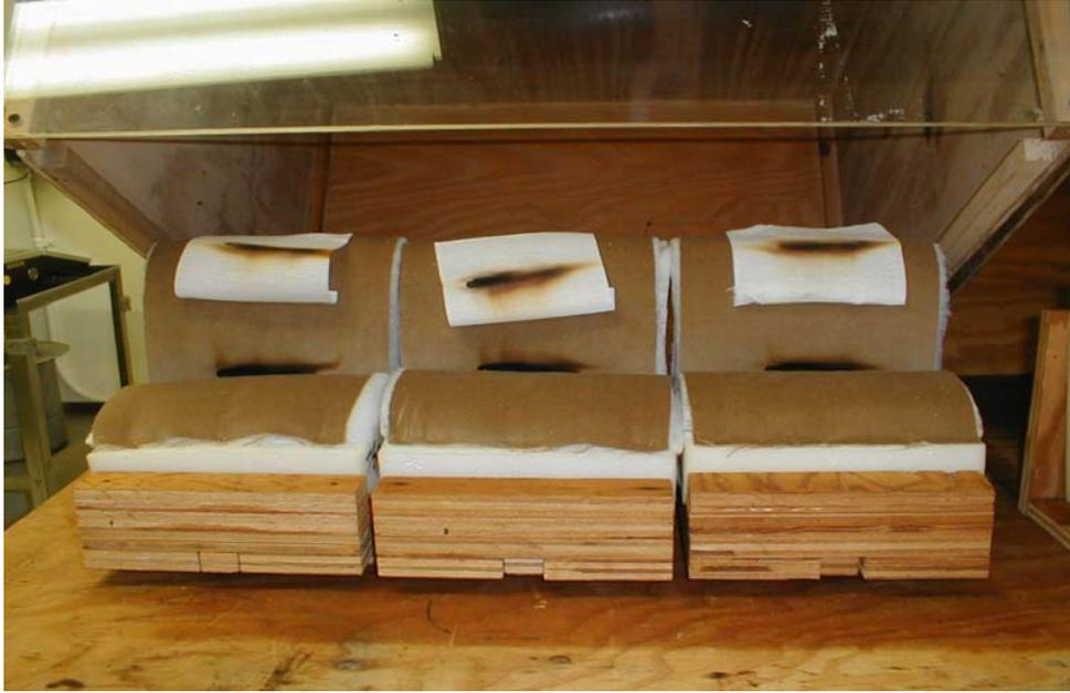
Figure 16 (a). Post Test Mockups of Fabric 24 with Foam U and UFAC Polyester Batting (top)/Interliner V (under)
