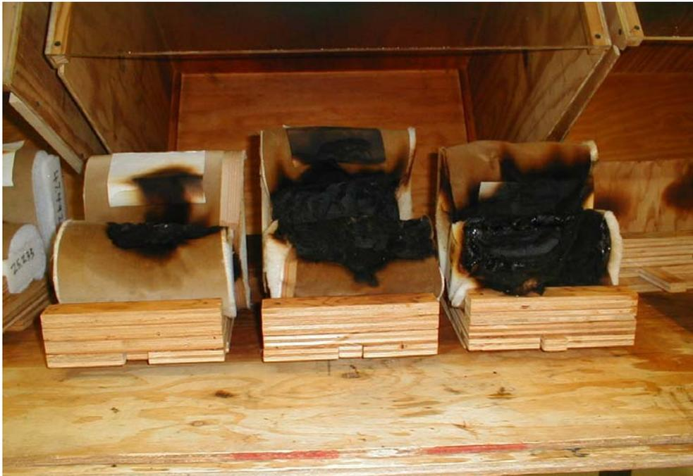
Figure 16 (b). Post Test Mockups of Fabric 24 with Foam U and Interliner V (top)/UFAC Polyester Batting (under)
