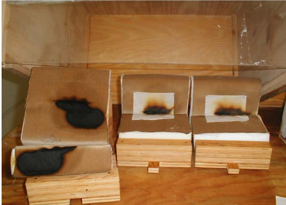
Figure 34. Post Test Mockups of Fabric 24 with Foam U and Interliner V
