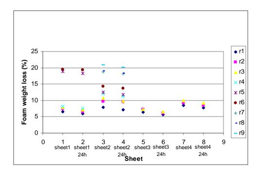
Figure 2. Fabric 24 Foam T Weight Loss with and without 24 hour Reconditioning
