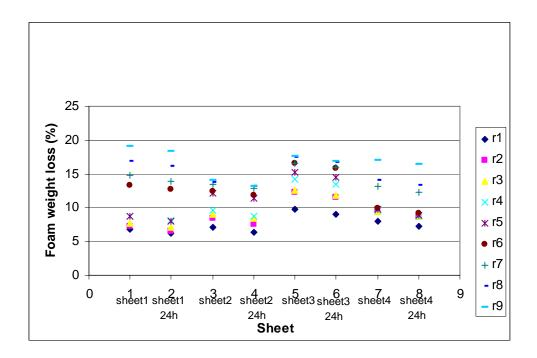
Figure 1. Fabric 23 Foam T Weight Loss with and without 24 hour Reconditioning
