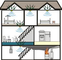
Single-Station Smoke Alarms Interconnected Smoke Alarms Wireless Interconnected Smoke Alarms
