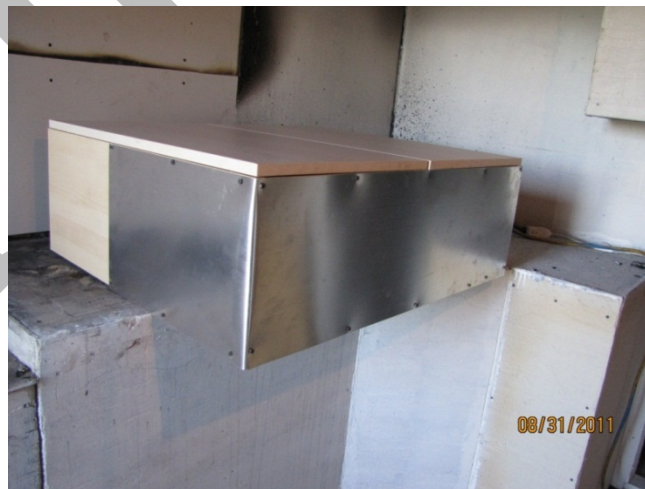
Figure 8. Sheet metal barrier on bottom and side of wall cabinet.
