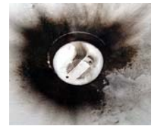
Figure 5. Soot ring around the alarm
