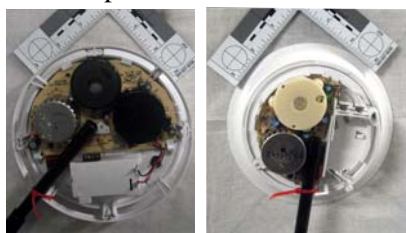
Figure 7. Ignition setup (cover removed for detail)
