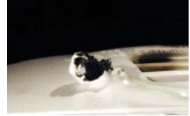
Figure 8. Capacitor shell lodged in the housing
