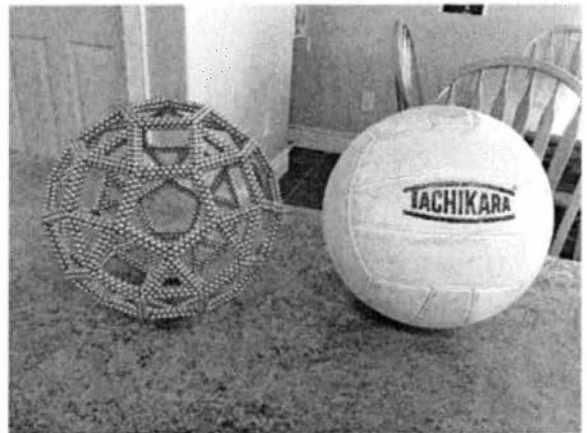
FIG. 30. Photograph of a hollow spherical rhombicosidodecahedron frame designed and built by the author using 3660 Zen Magnets. This structure barely supports itself under Earth's gravity, and cannot be built using weaker magnets.
