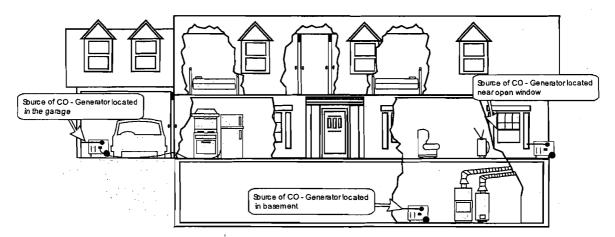
Figure 2. Portable generator located in confined spaces or near an open window
