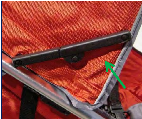
Figure 14a. Canopy stretcher (arrow). Fig. 14b. Hazardous method to secure canopy rod.
