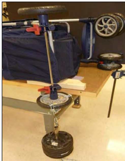
Figure 10. 100 lbm. suspended from wheel while stroller is secured to a workbench.
