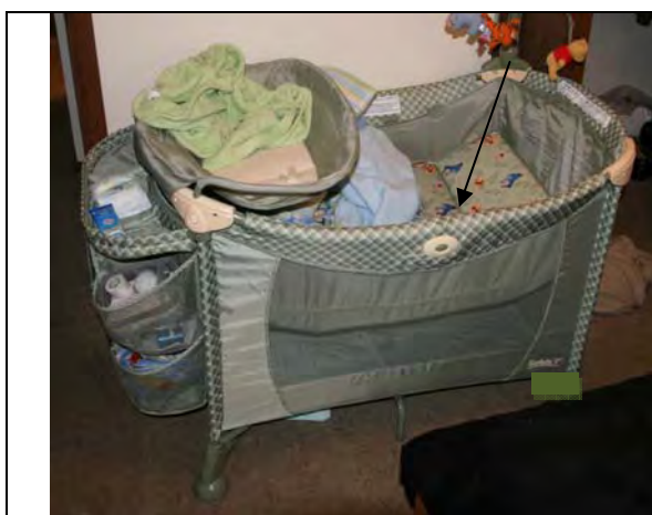
Figure 5. Incident bassinet play yard – photo from in-depth investigation (arrow pointing to V-angle in the mattress pad)
