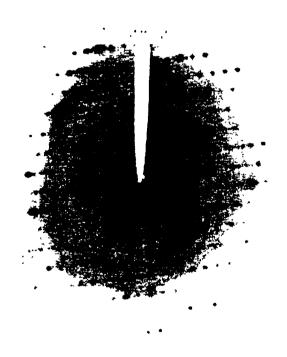
Image of anthophyllite fiber, F22, and its Selected Area Diffraction Pattern showing [121] Zone Axis; Mg:Si ratio of this fiber is 6.74:8.
