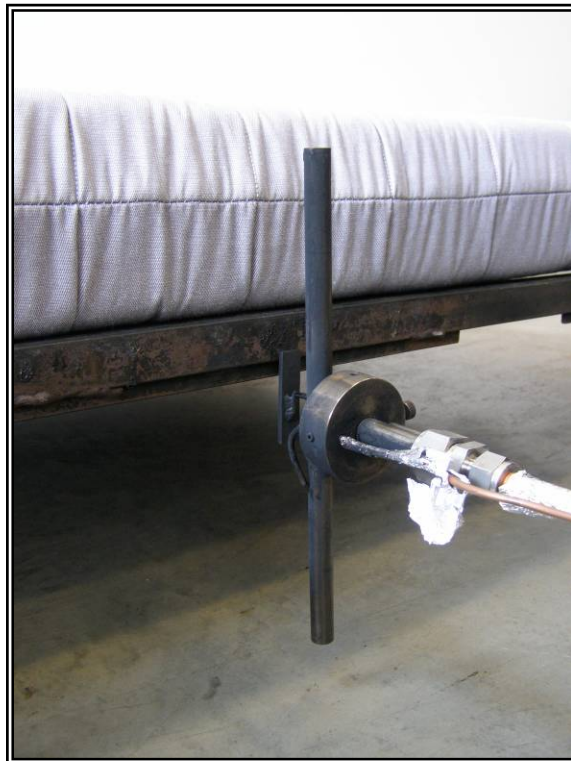
Figure 35. 16.1 Alignment of the side burner for thin specimens.
