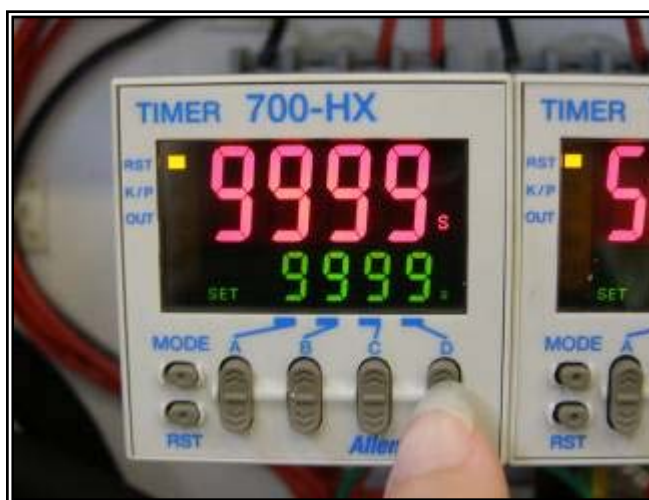
Figure 46. Step 5 Timer set to maximum time
