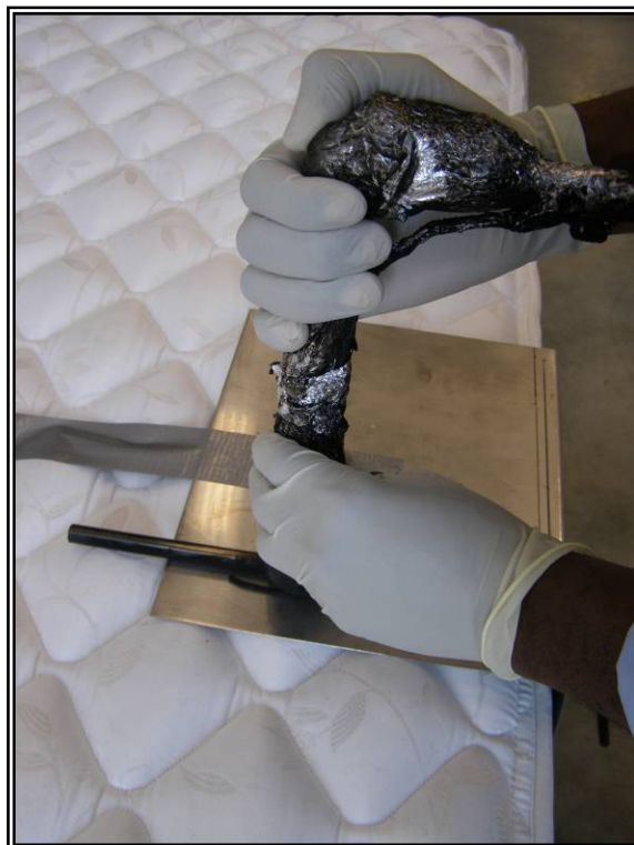
Figure 18. Step 14 Make burner face parallel to platen.
