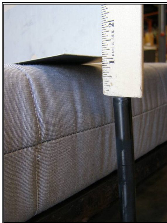
Figure 36. 16.1 Side burner one inch below top of specimen.
