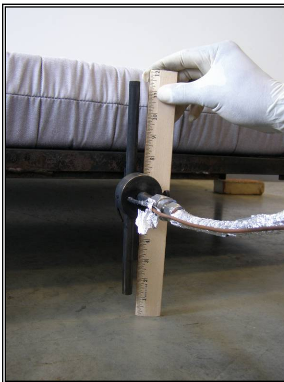
Figure 37. 16.1 Side burner one inch above test floor.
