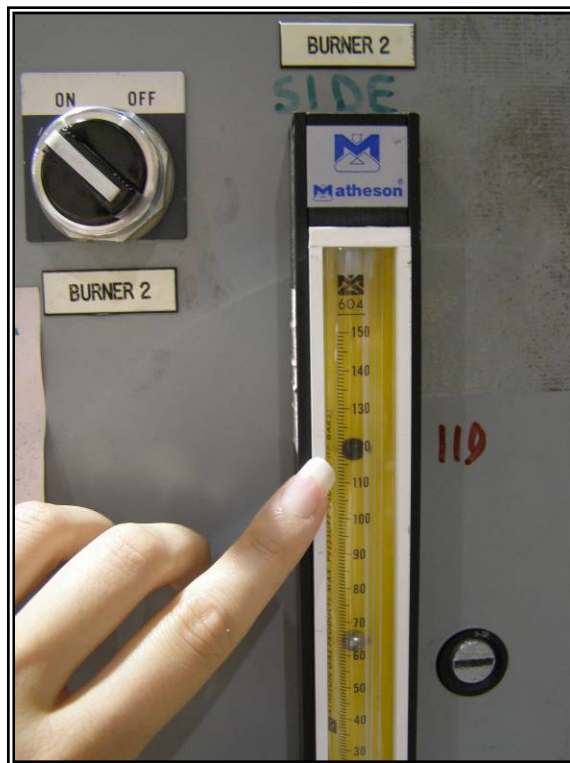
Figure 34. Step 38 Check flow rates.
