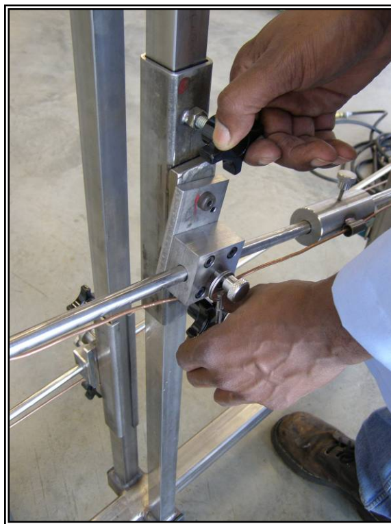
Figure 17. Step 13 Adjust top burner height.
