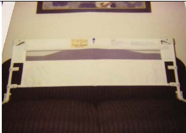
1. Bed rail incompletely assembled without middle bar Ref: IDI 050324HCC1605 (Criteria 6.9.1)
