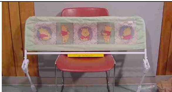
3. Bed rail misassembled - fabric cover does not engaging the bottom bar. Ref: 030730HCC1771 (Criteria 6.9.3)
