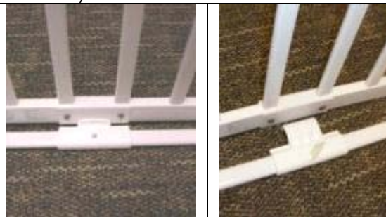
4. Bed rail misassembled - upside down placement of critical assembly component (right picture) (Criteria 6.9.4)
