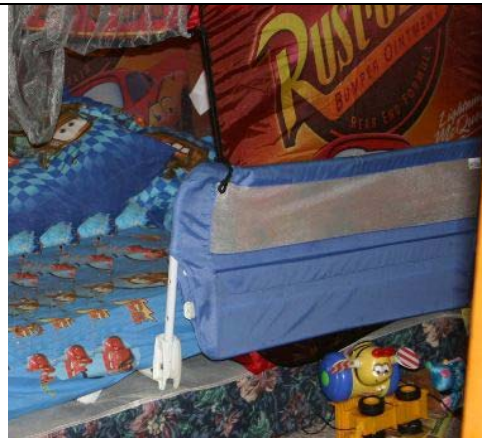
2. Bed rail misassembled without the middle bars attached to the end post. This is a misassembly because the screws were not use. Ref: IDI 080925HCC2061. (Criteria 6.9.2)
