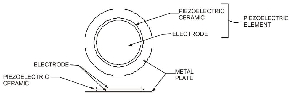
Figure 1. Piezoelectric Diaphragm
