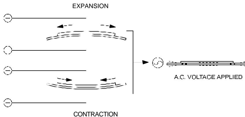
Figure 2. AC Voltage Applied to the Piezoelectric Element
