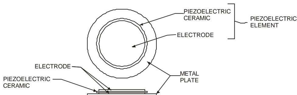
Figure 1. Piezoelectric Diaphragm
