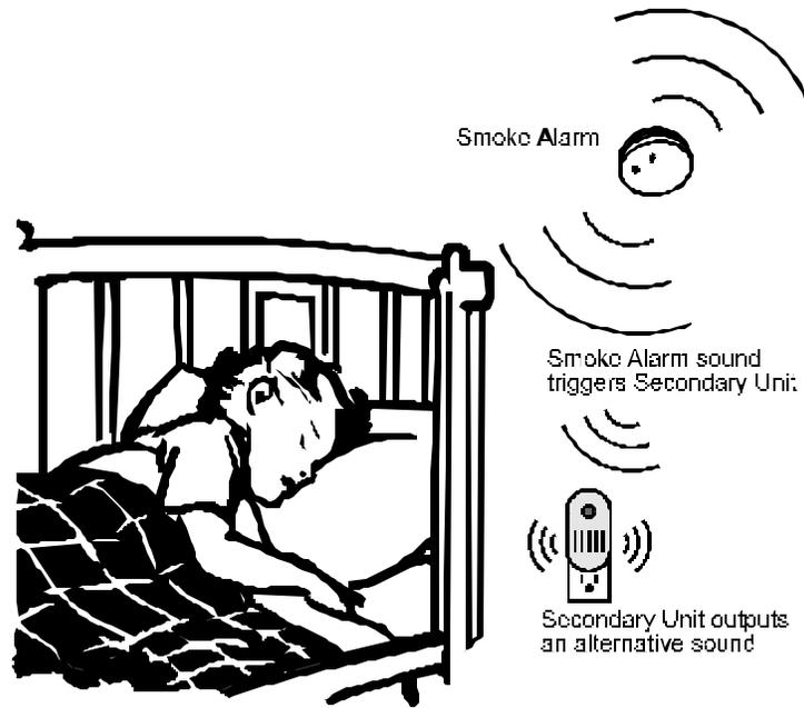
Figure 7a. Secondary Unit Triggered By Smoke Alarm Sound
