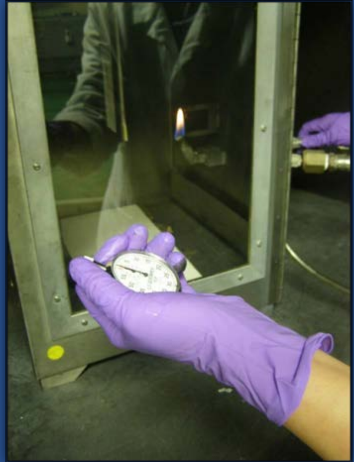
Preparing to apply ignition source to specimen
