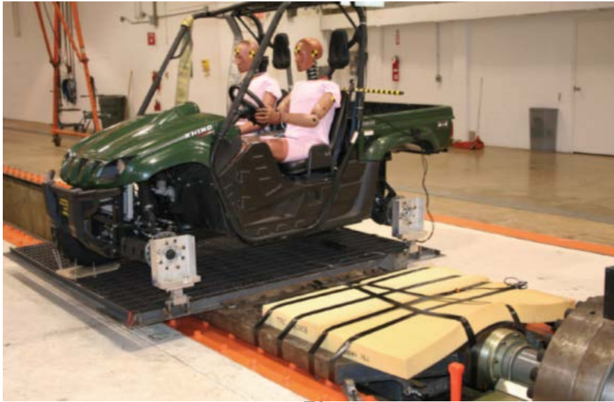
Figure 7: HYGE™ sled test set-up.
