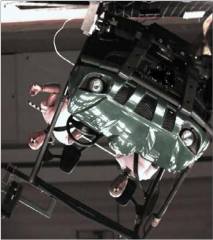
Figure 17. Belted occupant test using HYG TM sled test device.
