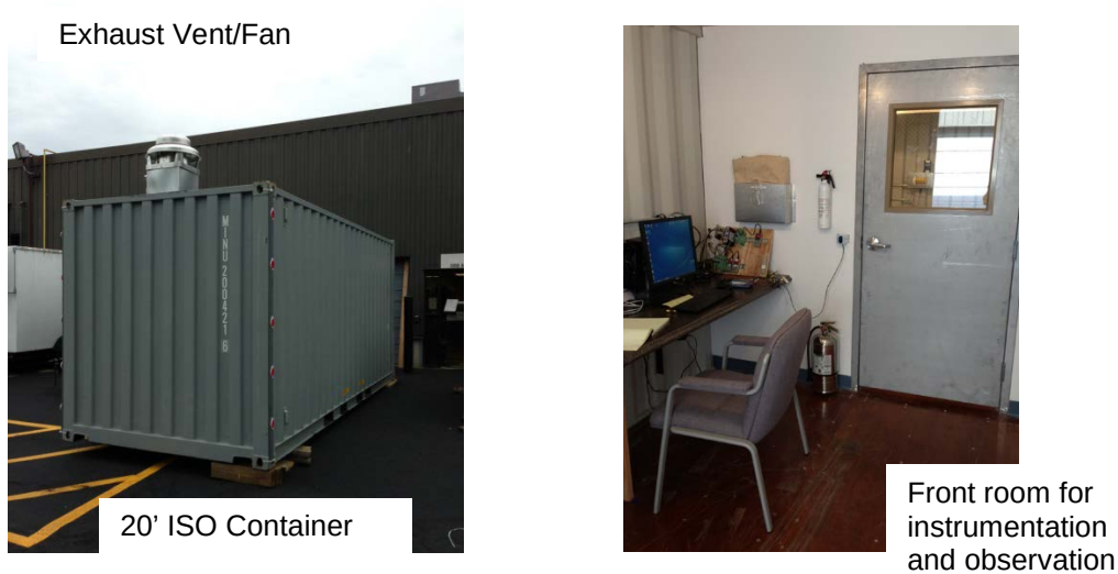
Figure 1: Outside and Inside Cooktop Fire Test Facility
