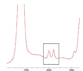
**Figure 1.** IR spectrum of PVC plastic containing ~30% phthalates.
