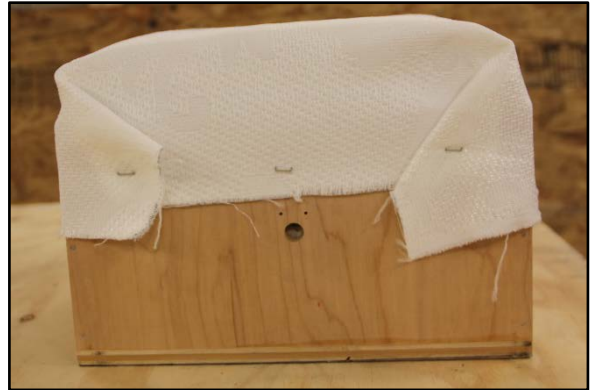
Figure 27. Ticking fastened, using staples.
