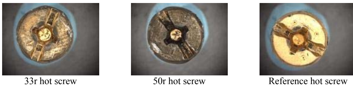
Figure 8: Comparison of the appearance of hot screws from receptacles harvested from components 33 and 50 to the appearance of a reference hot screw (never installed in a home).
