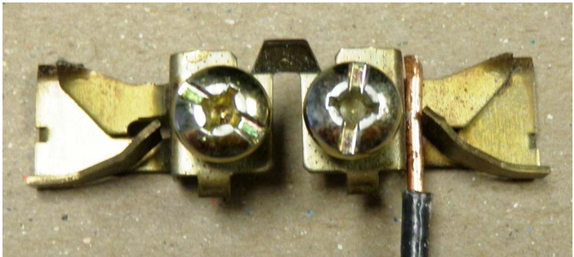
Figure A3. Receptacle terminal removed to show how a BWPI connection is formed.
