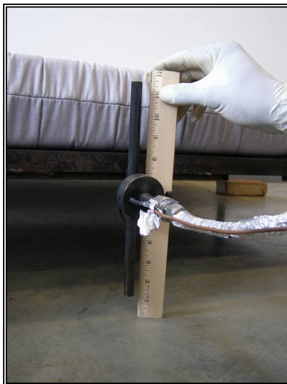
Figure 37. 16.1 Side burner one inch above test floor.
