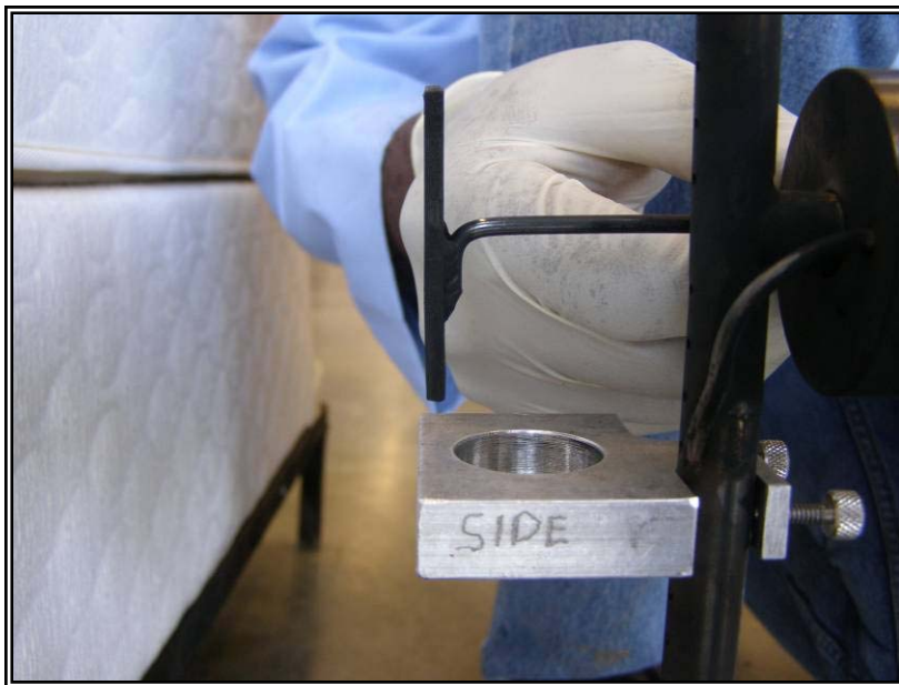
Figure 25. Step 21 Set stand-off foot distance with jig.
