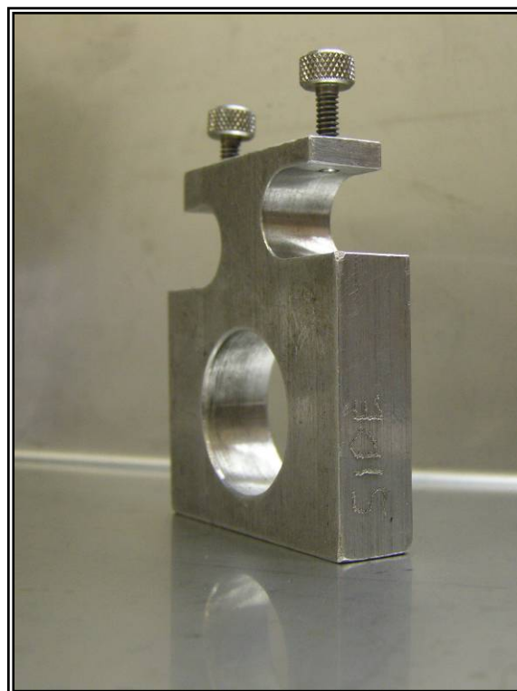
Figure 39. Burner stand-off foot jig
