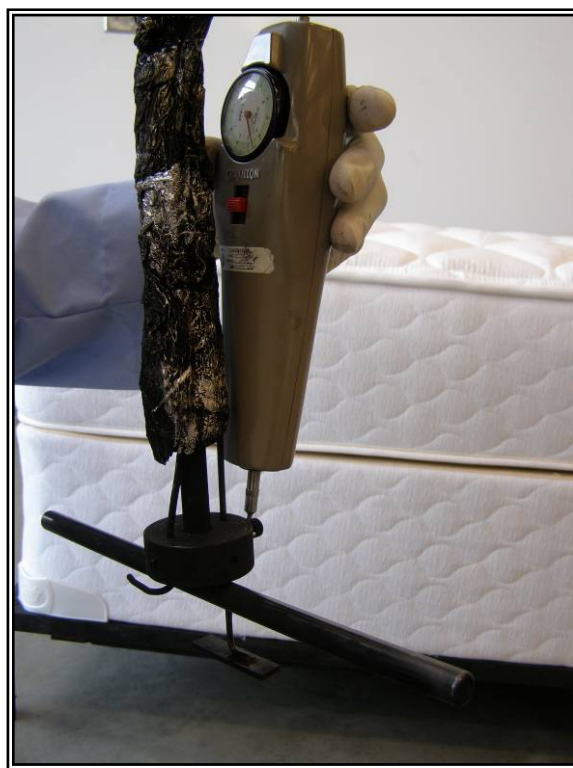
Figure 27. Step 23 Measure downward force using spring scale.
