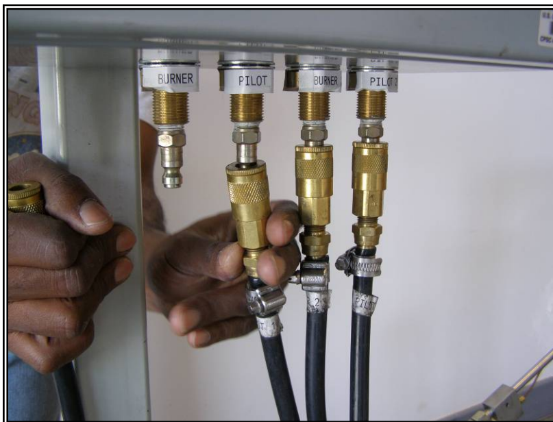
Figure 10. Step 3 Connect hoses to control box.
