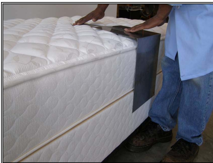
Figure 14. Step 10 Secure the platen.
