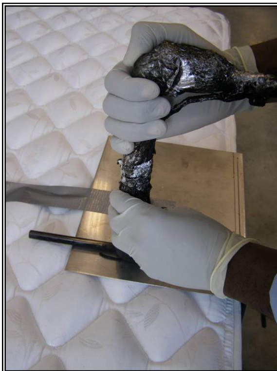
Figure 18. Step 14 Make burner face parallel to platen.
