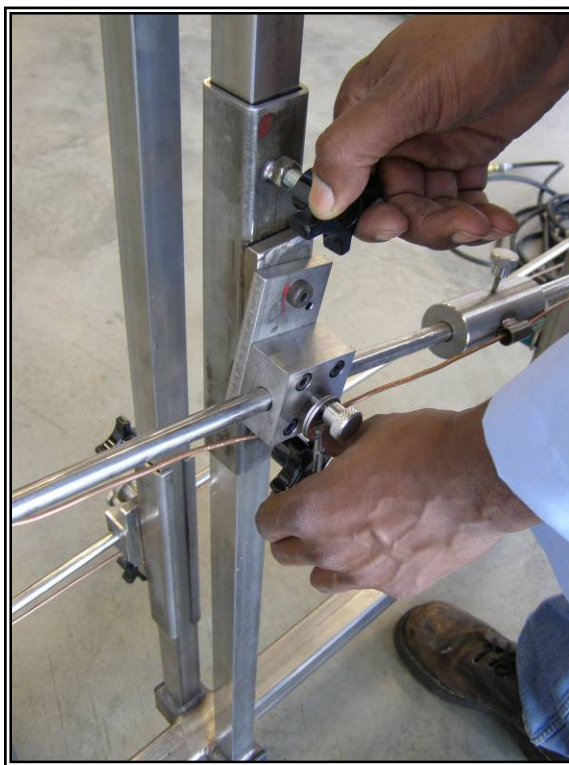
Figure 17. Step 13 Adjust top burner height.
