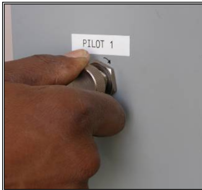
Figure 12. Step 10 Set pilot flow.
