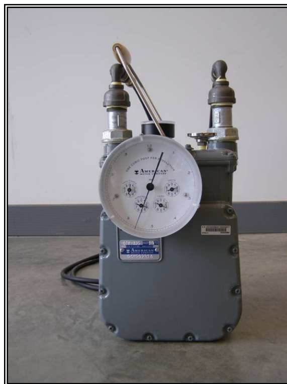
Figure 40. Diaphragm-type test meter
