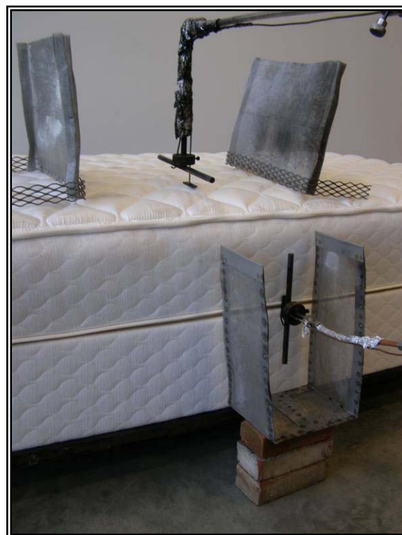
Figure 32. Step 35 Screens placed around burners.
