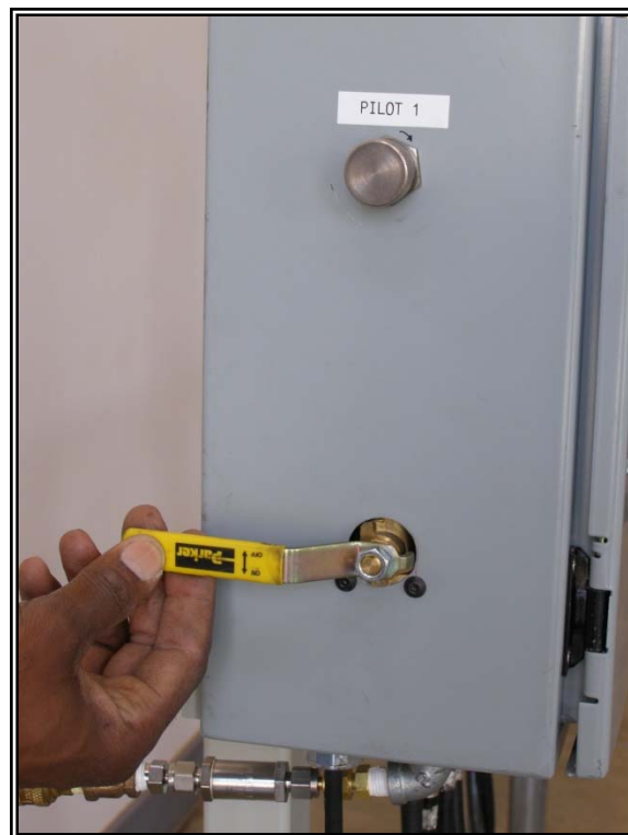
Figure 31. Step 32 Open pilot ball valves.
