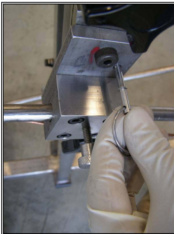
Figure 26. Step 22 Remove pivot point pin.
