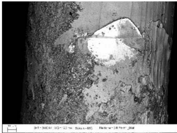
Figure 59. SEM images of the hot wire from the receptacle in Circuit 3. The connection was a push-in connection. The contact point is shown in the image on the left. The image on the right shows a region of a hot wire that was covered by insulation on the bottom.
