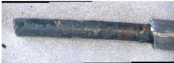
Figure 53. Optical images of wires from the standard receptacle from Circuit 3. Both the (A) hot and (B) neutral wire are shown. Both are “push-in” type contacts.
