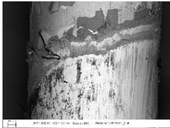
Figure 59. SEM images of the hot wire from the receptacle in Circuit 3. The connection was a push-in connection. The contact point is shown in the image on the left. The image on the right shows a region of a hot wire that was covered by insulation on the bottom.
