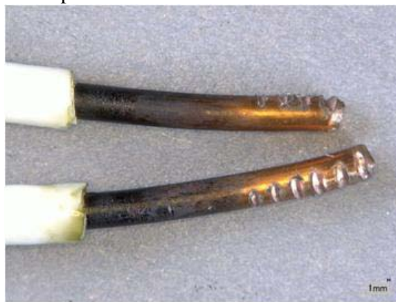
Figure 61. Optical images of twist-on connectors with hot and neutral wires used on the output section of Circuit 2.
