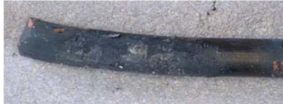
Figure 53. Optical images of wires from the standard receptacle from Circuit 3. Both the (A) hot and (B) neutral wire are shown. Both are “push-in” type contacts.
