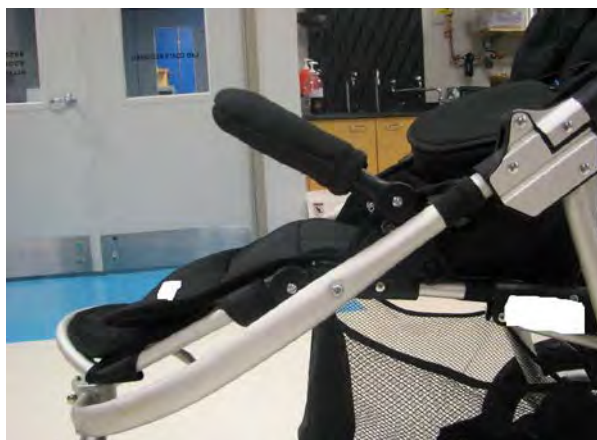
Figure 2. Grab bar in the car seat attachment position. The opening between the grab bar and seat FAILS ASTM F833-13b, Section 7.12, Passive Containment/Foot Opening Test Method .
