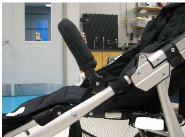
Figure 1. Grab bar in manufacturer-use position for an occupant. The opening between the grab bar and seat PASSES ASTM F833-13b, Section 7.12, Passive Containment/Foot Opening Test Method .
