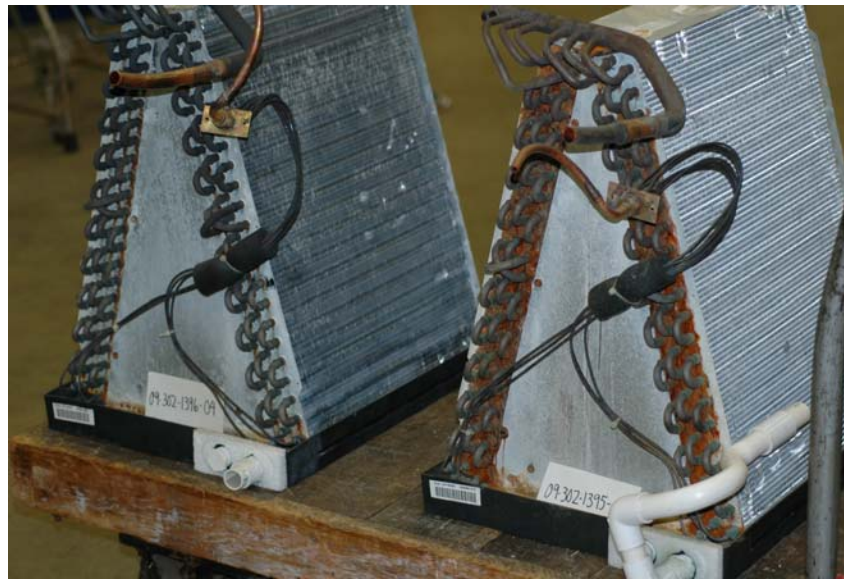
Figure 3 – Photograph of the two air conditioner evaporator coils showing the black discoloration of the copper U-bends and corrosion of the end plate.
