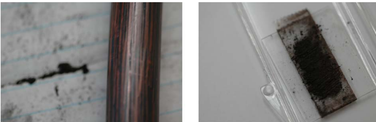
Figure 5 – Photographs of the scraped copper natural gas supply line and the slide holding the sample for X-ray diffraction.
