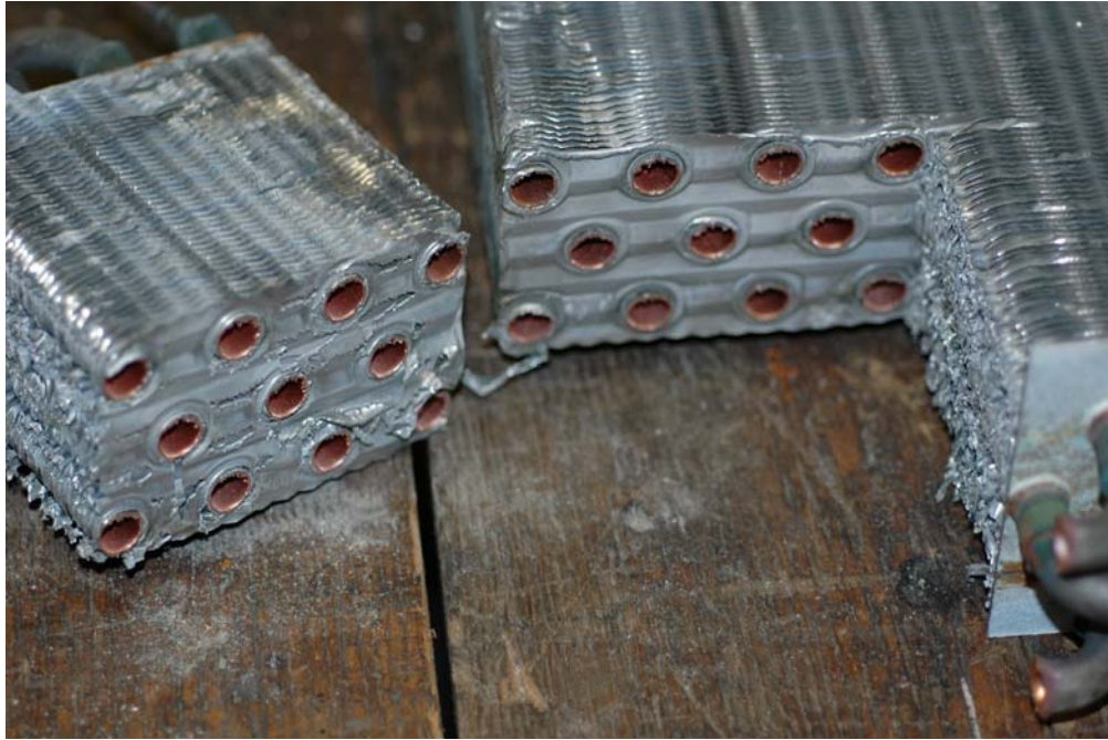
Figure 8 – Air conditioner evaporator coil after slicing to allow for examination for corrosion damage between the aluminum sheets and the copper tubing.
