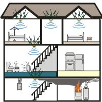
Interconnected smoke alarms are typically connected using a wire, but newer wireless technology is available that allows smoke alarms to be interconnected without using wires. This allows easier and less costly upgrade to interconnected smoke alarms for older homes. Not all homes may need interconnected smoke alarms. Small, single-level homes may not benefit from interconnected smoke alarms because of the close proximity between smoke alarms.
