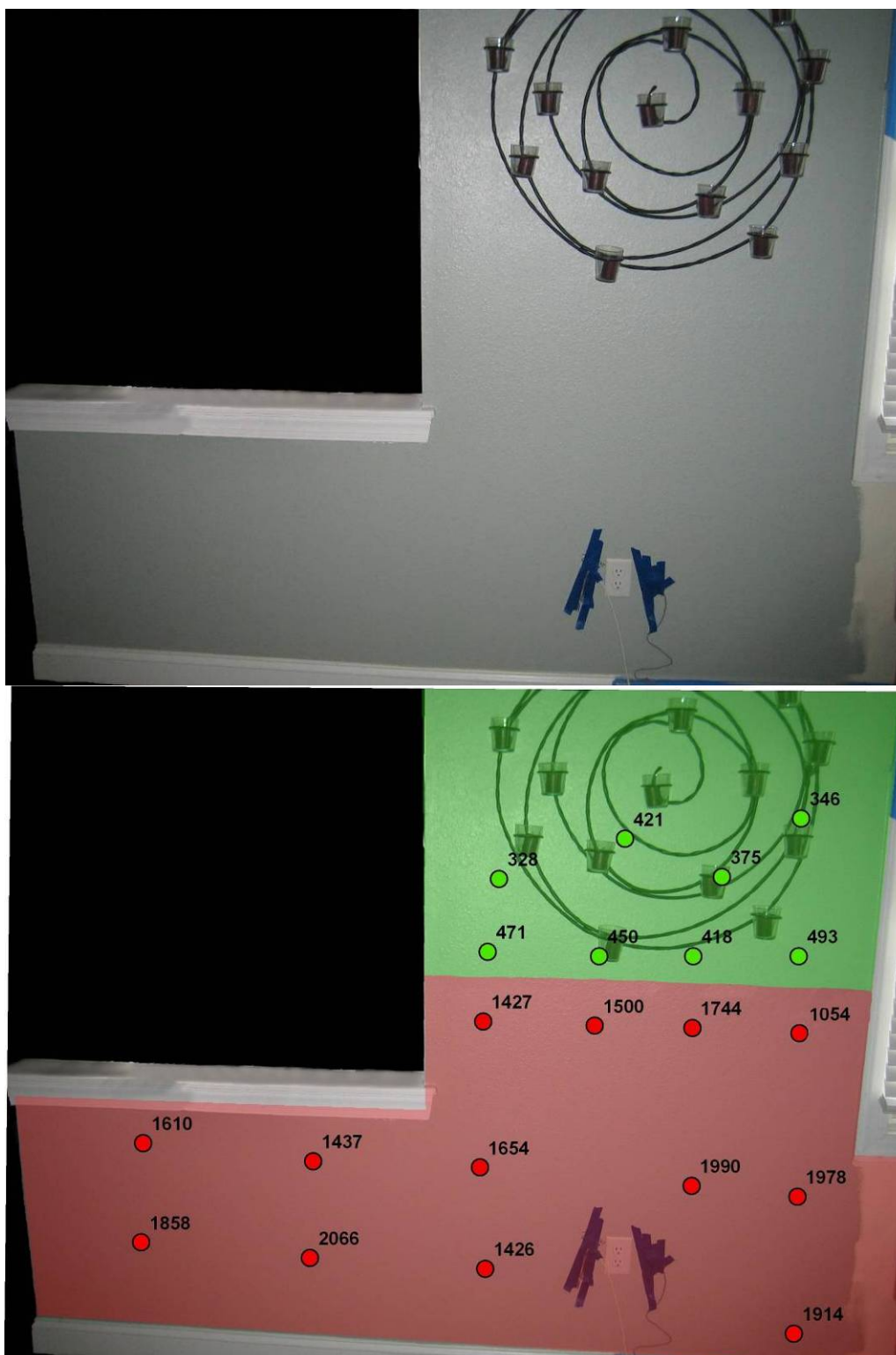
Figure 6.2 Picture of One Wall from a Complaint Home (a) and Same Wall with Strontium Concentrations Measured using XRF through Paint (b) demonstrating two Different Drywall Boards in an Otherwise Uniformly Painted Wall
