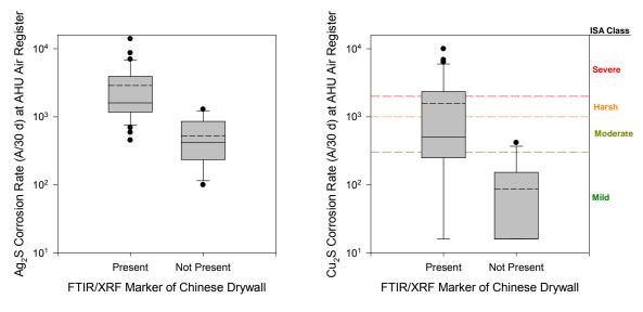
Figure 5.24 Comparison of Corrosion Film Thickness by FTIR/XRF Marker
