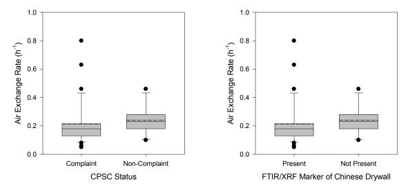
**Figure 5.17** Comparison of Short-term, House Average Air Exchange Rates by CPSC House Status and FTIR/XRF Status
