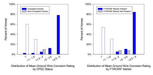
Figure 5.9 Comparison of Mean Ground Wire Corrosion Rating by CPSC Home Status
