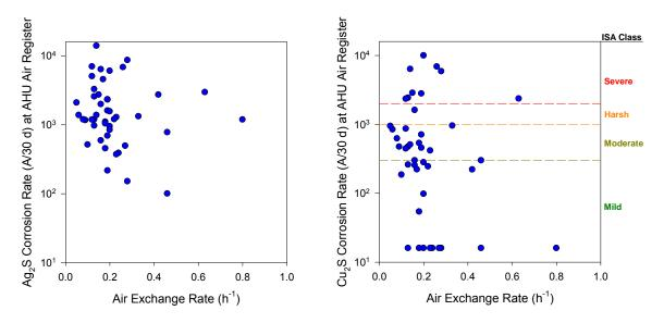
**Figure 5.18** Comparison of Corrosion Film Thickness at the AHU Air Register by Air Exchange Rate
