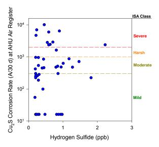
**Figure 5.14a** Comparison of Corrosion Rates at the AHU Air Register by House Average Hydrogen Sulfide Concentration Measured Using 2-week Passive Monitors
