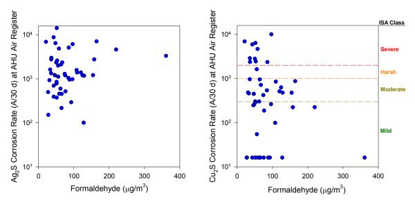
Figure 5.12 Comparison of Corrosion Film Thickness by Formaldehyde Concentration
