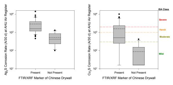
Figure 5.8 Comparison of Corrosion Film Thickness by FTIR/XRF Marker
