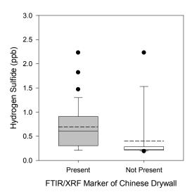
**Figure 5.21** House Average Hydrogen Sulfide Concentration (ppb) by a) CPSC House Status, and b) FTIR/XRF Marker
