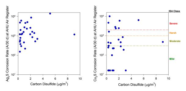
**Figure 5.16** Comparison of Corrosion Film Thickness at the AHU Air Register by House Average Carbon Disulfide Concentration
