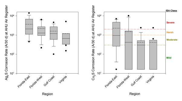
Figure 5.10 Comparison of Corrosion Film Thickness Across Study Regions
