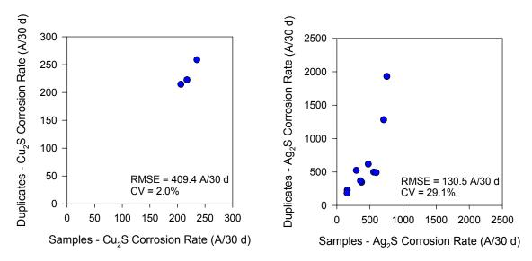
**Figure 4.6** Comparison of Paired Duplicate Corrosion Rate Measurements for Copper and Silver Coupons
