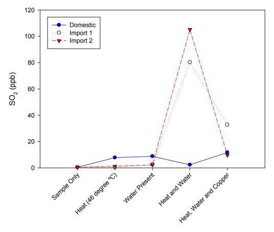
**Figure 6.5** Sulfur Dioxide (SO<sub>2</sub>) Concentrations inside Small-volume Chamber Studies Comparing Two Imported and One Domestic Drywall Sample Under Varying Environmental Conditions.
