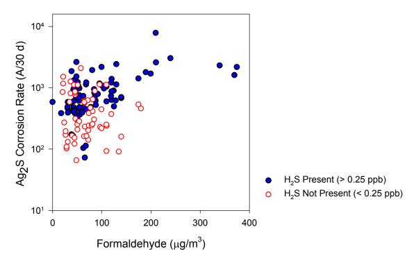
**Figure 5.25** Scatterplot of Silver Corrosion Rate by Indoor Formaldehyde Concentration, Stratified by the Presence or Absence of Hydrogen Sulfide
