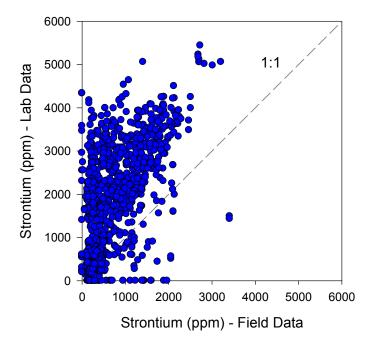
**Figure 6.3** Comparison of Strontium Concentrations of Co-located Samples Measured in the Field through Paint and/or Plaster, and Samples Measured of the Drywall Core in a Controlled Laboratory Setting
