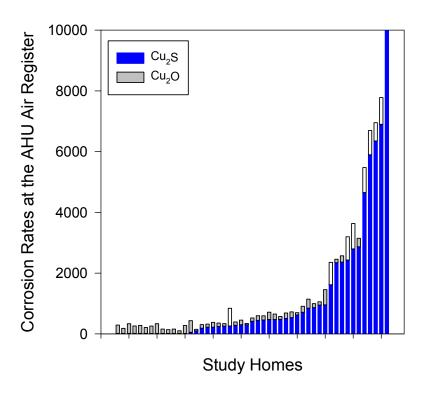
Figure 5.5 Corrosion Rates at AHU Air Register for All 51 Homes, by Corrosion Species
