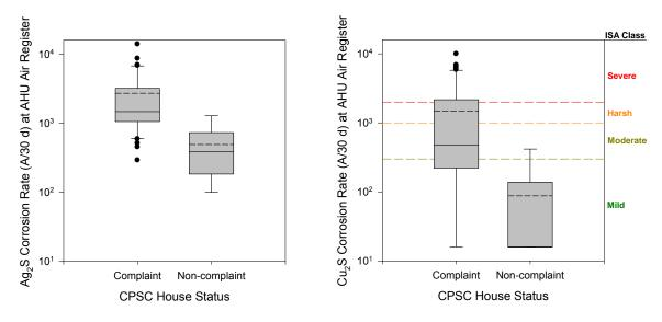
Figure 5.7 Comparison of Corrosion Film Thickness by CPSC House Status
