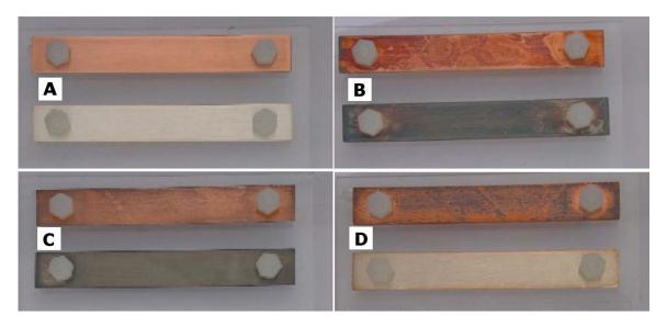
**Figure 5.4** Photographs of Corrosion Coupons after Retrieval from One Non-complaint Home (A) and Three Complaint Homes (B – D)
