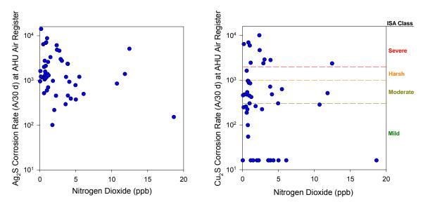
**Figure 5.14b** Comparison of Corrosion Rates at the AHU Air Register by House Average Nitrogen Dioxide Concentration Measured Using 2-week Passive Monitors
