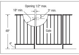
Use this as a guide when the release mechanism is located less than 54 inches from the bottom of the gate.
