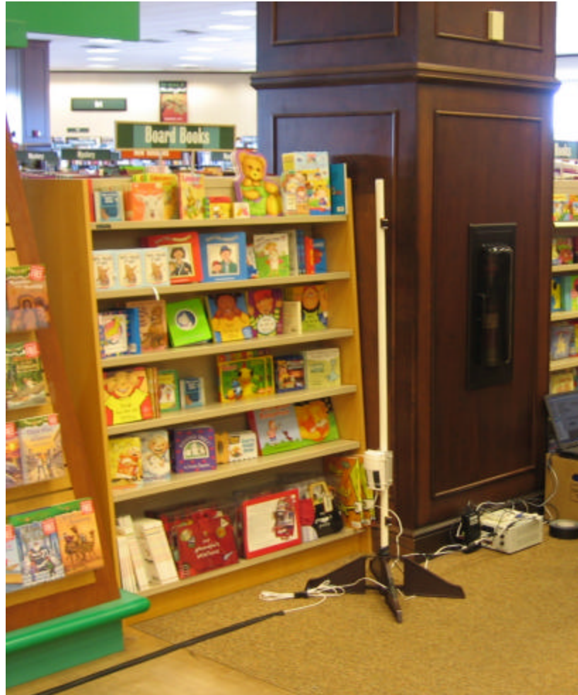
Figure 12: Detector Pole (with PIR Sensor) Position
