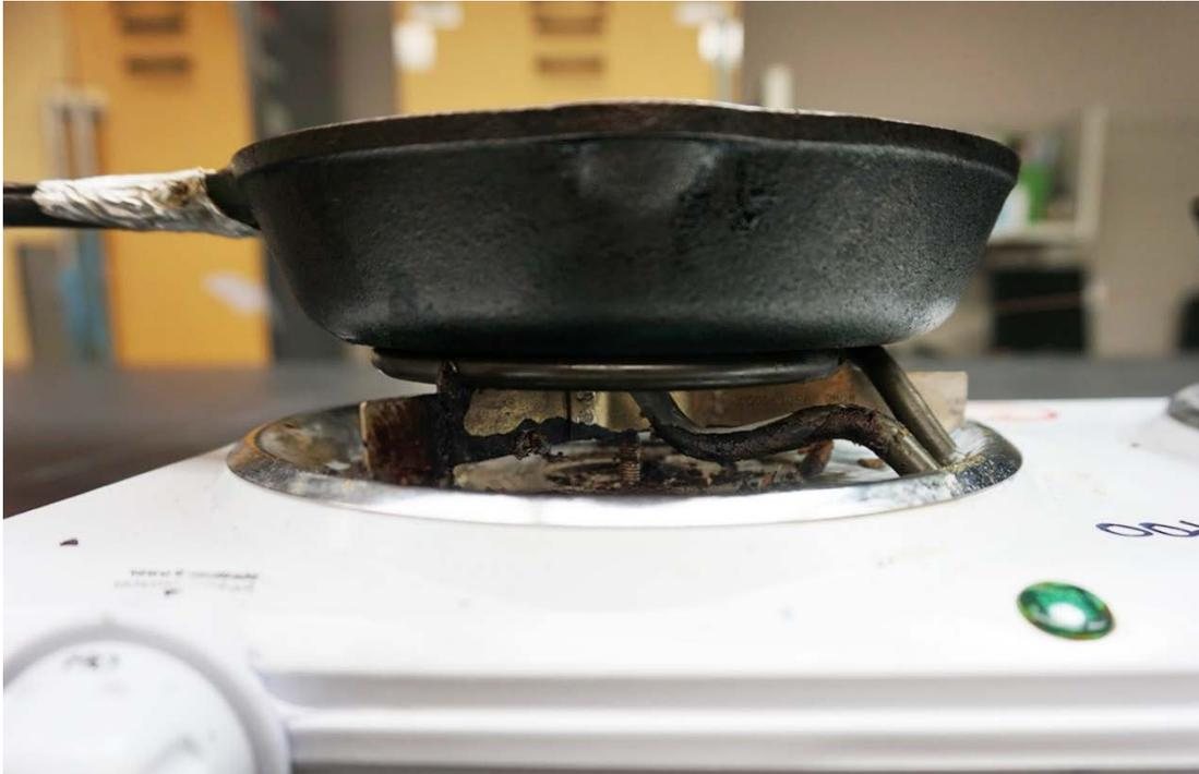
**Figure 10: 6" Cast Iron Pan on 4" (600 W) Element**
