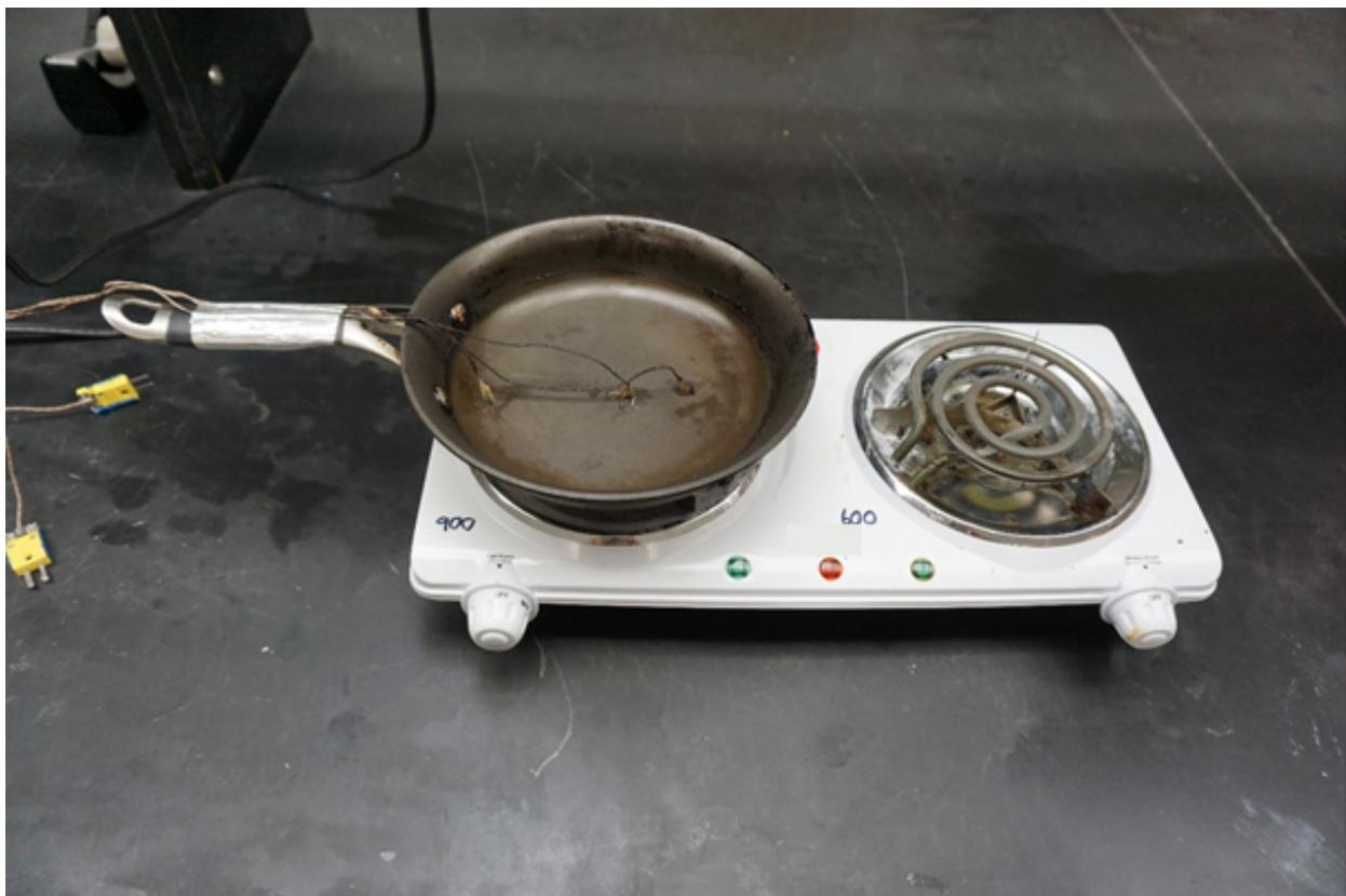
**Figure 7: 8" Aluminum Pan on 900 W (Rated) Coil Element**
