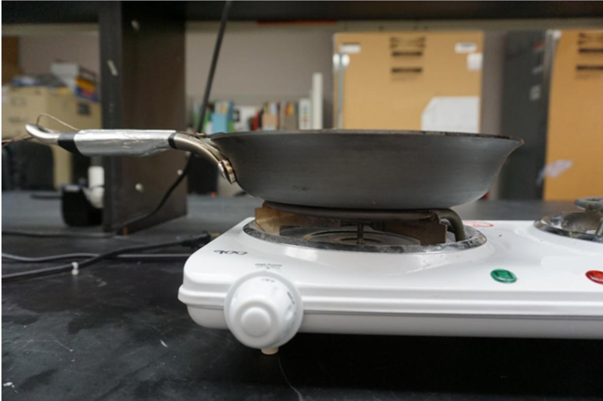
**Figure 8: Side View of 8" Aluminum Pan on 6", 900 W (rated) Coil Element**
