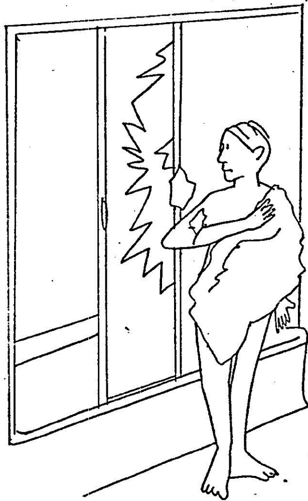
TUB ENCLOSE GLASS BREAKS RESULTING IN LACERATION
