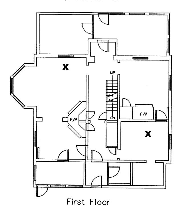
FIGURE 8. QUARTERS 'A' FIRST FLOOR SMOKE ALARM LOCATIONS
