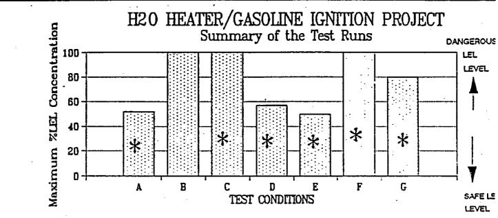
A: 6 in elevation / 2000 mL spill / Pilot cover off
