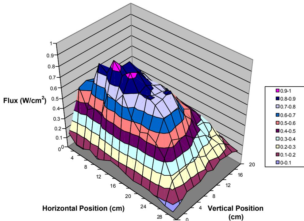
**Figure 7: Heater A Flux Map, Sensor Position = 2 cm from the Heater Front**
