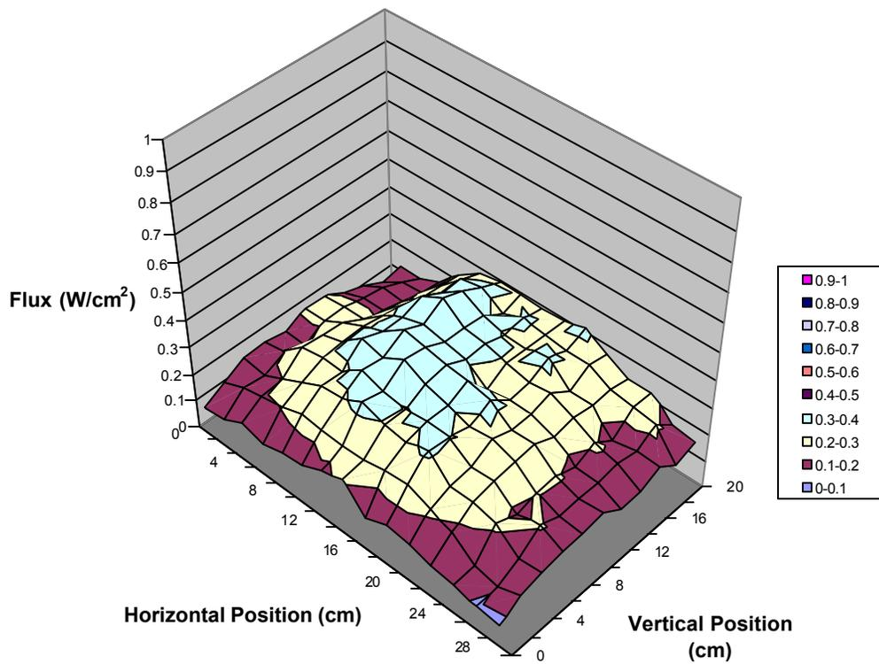
**Figure 9: Heater A Flux Map, Sensor Position = 10 cm from the Heater Front**
