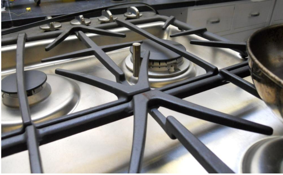
Figure 7: Side View of RTD Sensor Integrated with the Largest Burner of the Gas Cooktop
