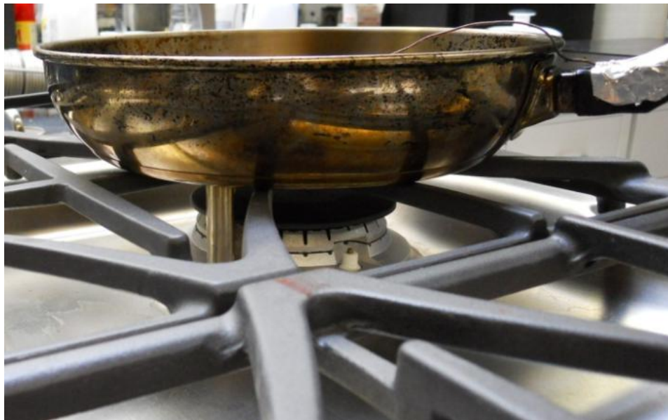
Figure 8: RTD Sensor Being Engaged by a Stainless Steel Pan
