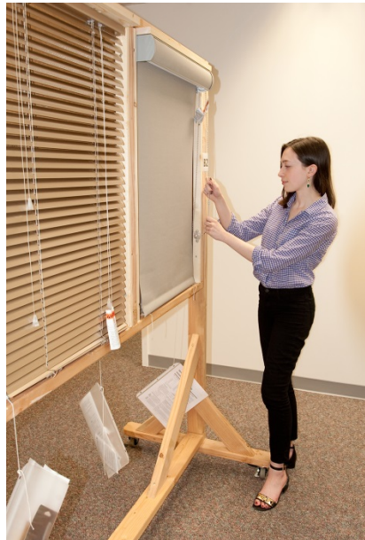
Figure 4. Analyst interacting with window covering in mounting apparatus
