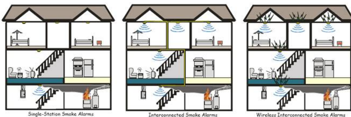
Figure 5: Interconnected Smoke Alarms (Consumer Product Safety Commission)
