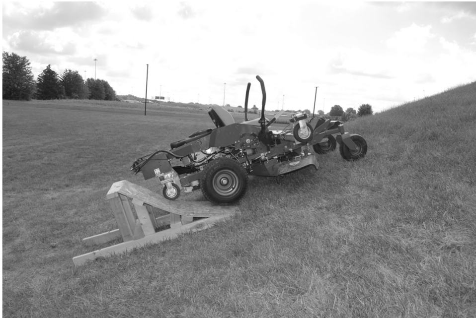
Vehicle C – Photo Sequence of Zero-Turn Mower Quasi-Lateral Tip-up
