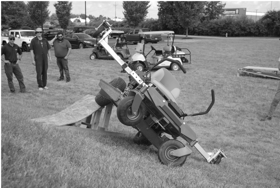
Vehicle C – Additional Photos of Zero-Turn Mower Quasi-Lateral Tip-up
