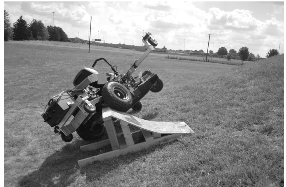
Vehicle C – Photo Sequence of Zero-Turn Mower Quasi-Lateral Tip-up
