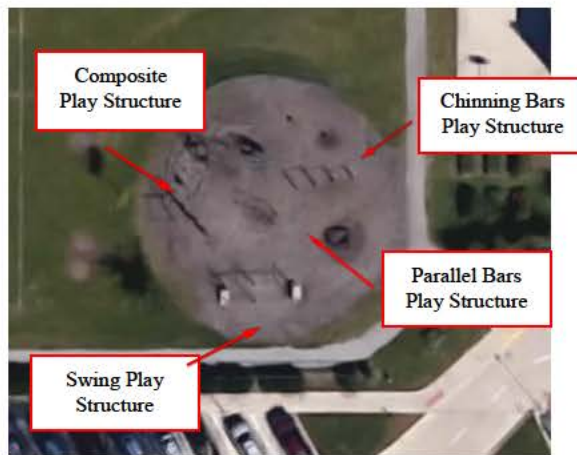
Figure A3. Impact attenuation test example with 4 structures, no overlapping use zones. Four structures requiring 3 test sites each with 3 drops at each test site for a total of 36 drops.
