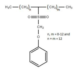
Figure 2. Secondary disulfonic acid phenyl esters
