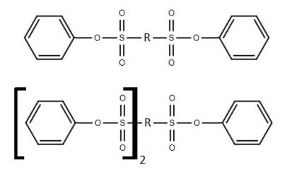
Figure 1. Di- and tri- esters of ASE (adapted from DEZA, 2013)
