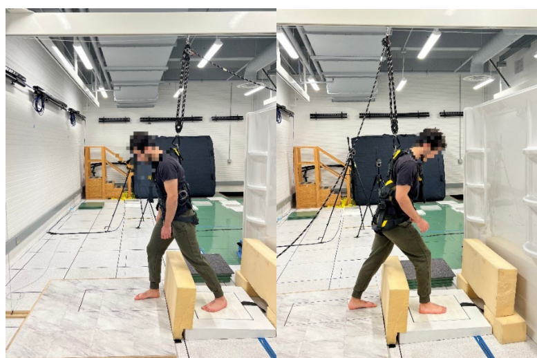
Figure 3A. Side-view showing “Bathtub” mockup used for subject testing (note: all dimensions in inches). Figure 3B. Side-view of the testing showing a participant entering and exiting the Bathtub mockup.
