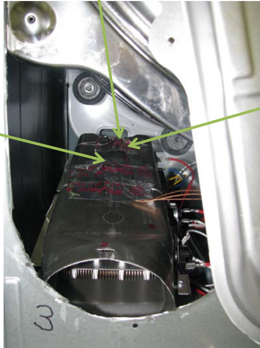
Figure A-16. Dryer 3: Locations of TC 24, 26, and 27.
