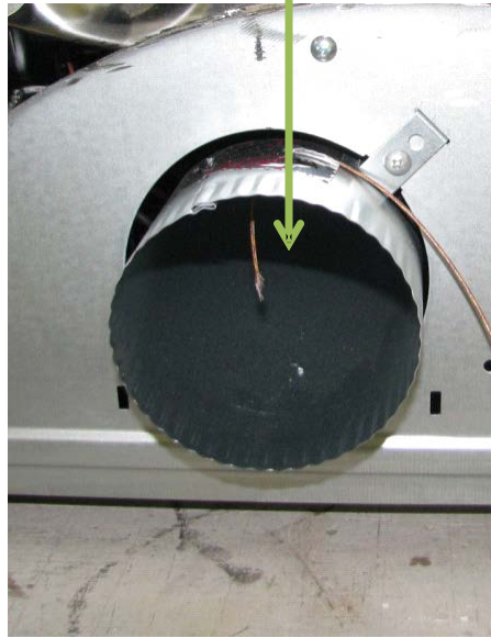
Figure A-18. Dryer 3: Location of TC 32.
