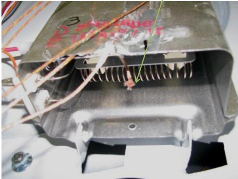
Figure A-2. Dryer 1: Location of TC 1.
