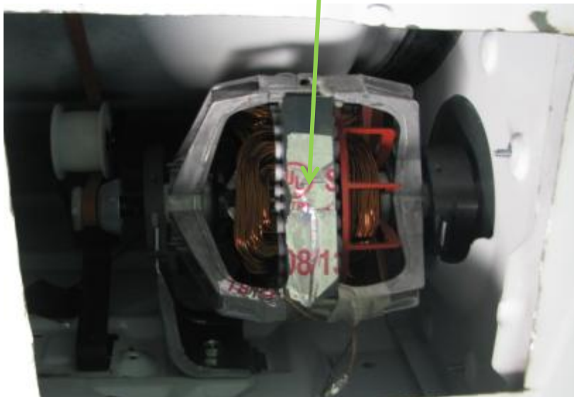
Figure A-5. Dryer 1: Location of TC 8
