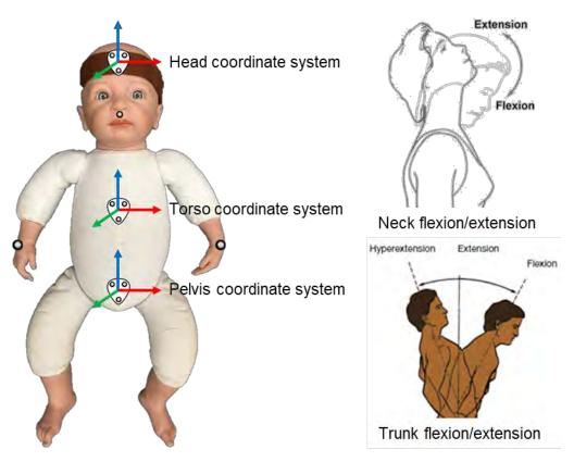
Figure 14. Infant body segment coordinate systems (L), and neck and trunk sagittal plane angles for which ranges of motion were calculated (R)
