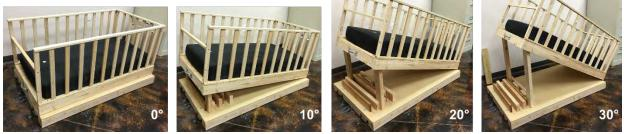
Figure 7. Photos of the four incline settings of the inclining crib
