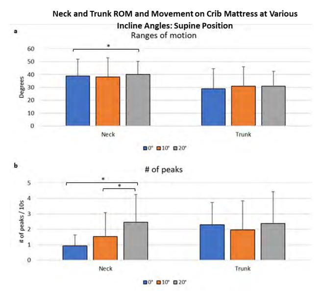
**Figure 20.** Effect of inclined crib mattress surface (0° vs. 10° vs. 20°) during supine positioning on (a) ranges of motion and (b) number of peaks [neck: number of times an infants raised their heads relative to their trunks; trunk: number of times infants raised their trunks relative to their pelvises]. \* p<0.05.
