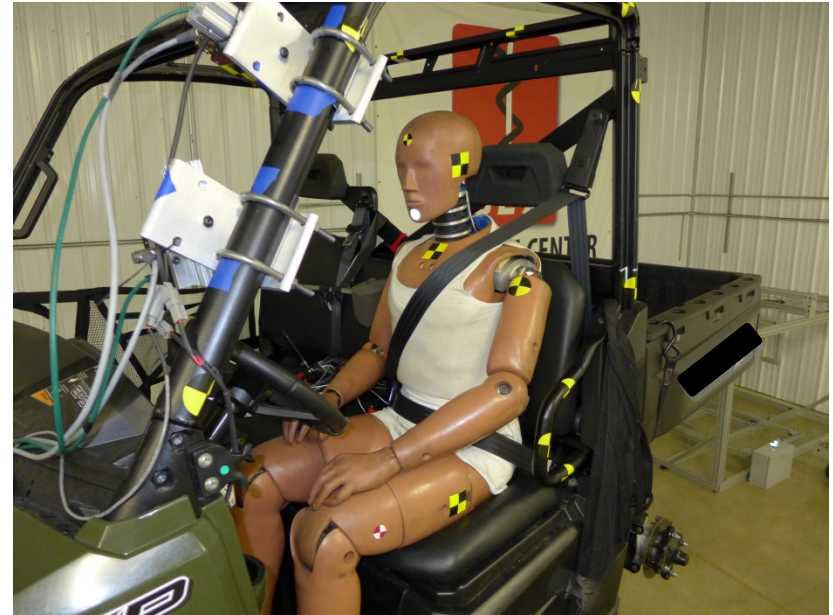
Figure 13: Vehicle L15 on the Roll Simulator - Additional Tests, Net Removed
