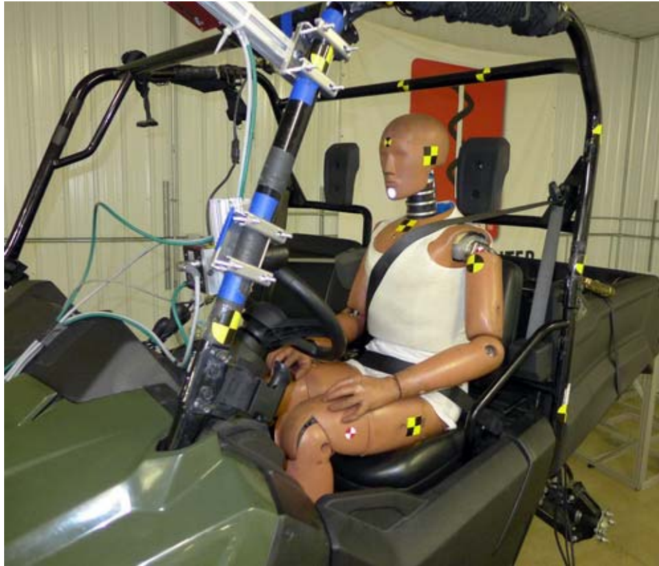
Figure 7: Vehicle J15 on the Roll Simulator - Additional Tests, Net Removed
