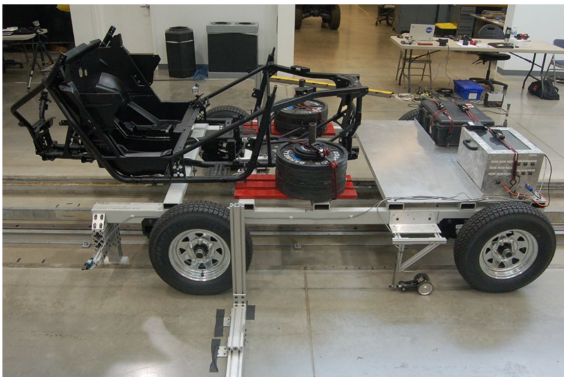
Figure 23: Sled Cart with OEM ROV Frame (Vehicle A) Attached
