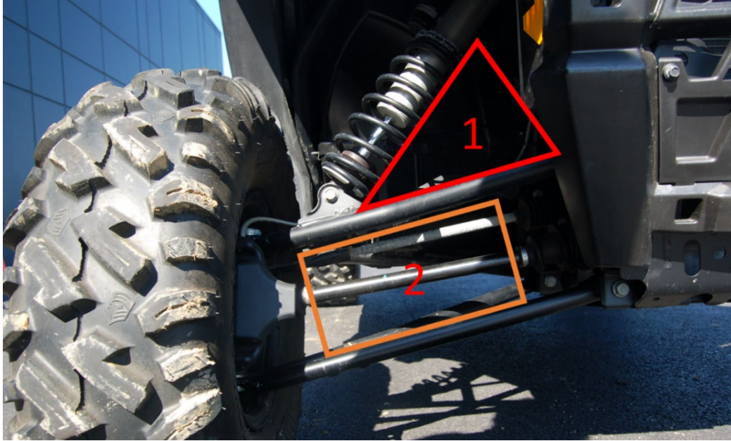
Figure 2: Two Stick Penetration Zones Used for Vehicle A.
