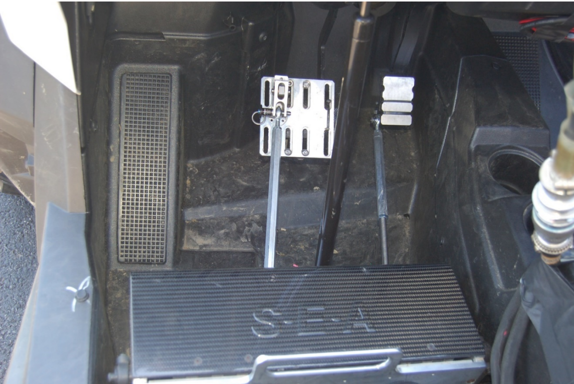
Figure 5: Brake and Throttle Robot Used to Control Vehicle Speed
