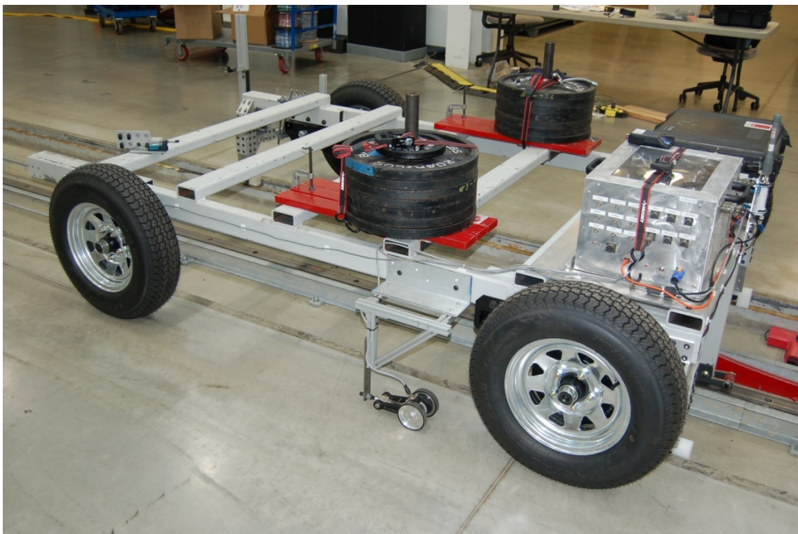
Figure 22: Sled Cart Used for ROV Debris Penetration Tests
