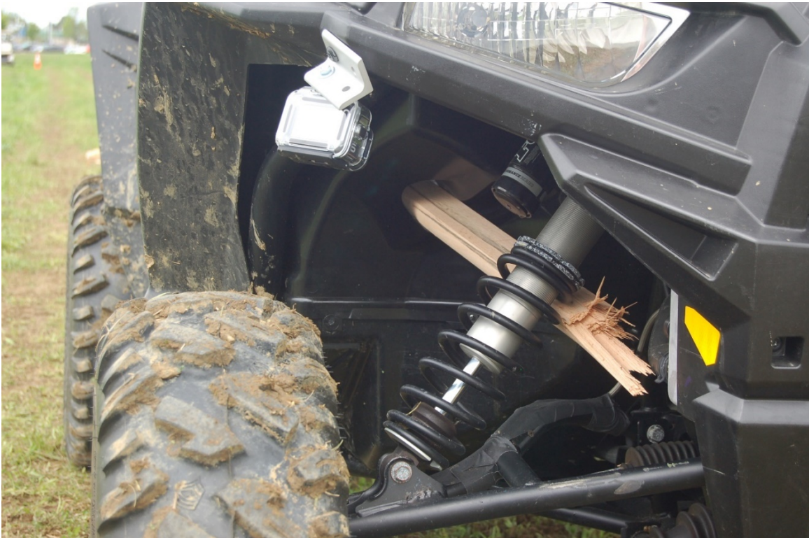
Figure 9: Run 1 Post-Impact Front View
