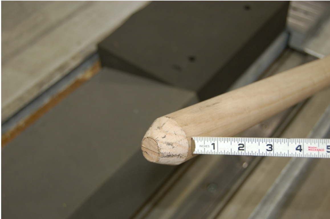
Figure 30: Taper on Impacting End of Stick.
