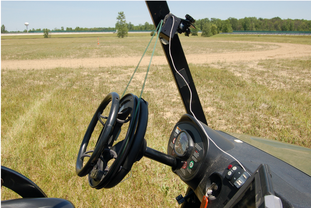
Figure 1: Steering Wheel Angle Sensor Mounted in Test Vehicle
