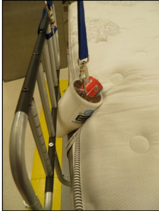
Figure 5: Demonstration of a product with a considerable gap between the mattress and the product (Zones 2 & 3).
