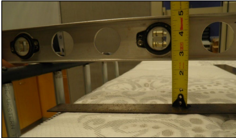
Figure 2: Demonstration of an APBR product failing the static height requirement in section 6.2.1.
