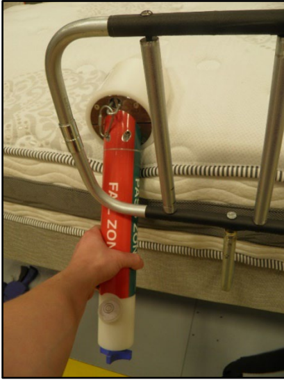
Figure 8: Demonstration of a structure that created a large opening at the ends of the rail.
