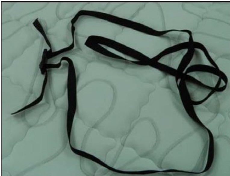
Figure 1: Example of a retention system that was not permanently attached to the product.
