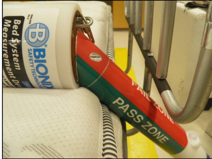
Figure 9: Demonstration of overhanging structure that is too high relative to the mattress.
