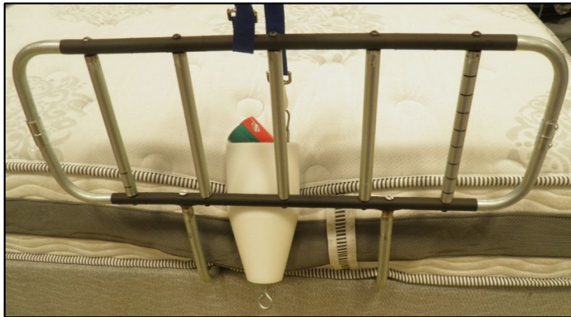
Figure 4: Demonstration of a product without sufficient internal structure to cover the Zone 2 opening.
