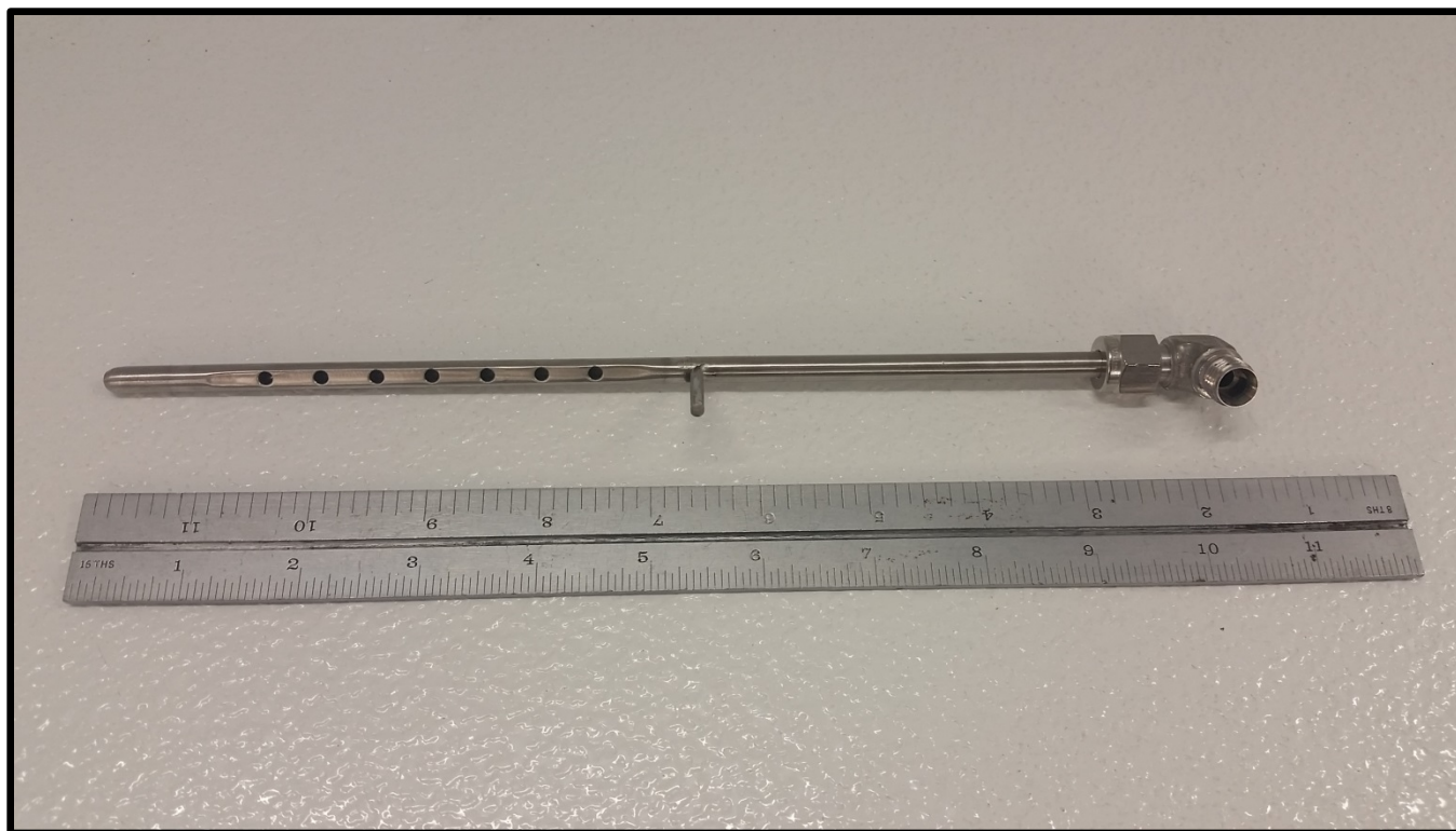
Figure 6. Nitrogen Injection Tube.
