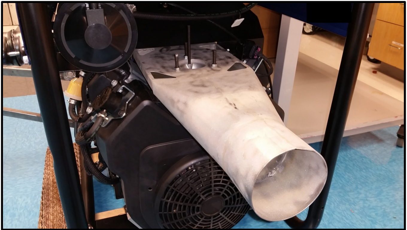
Figure 4. Dilution Tunnel Manifold for Test Engine
