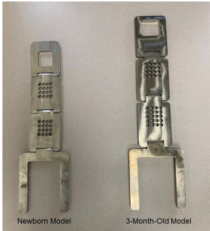
Figure 34. Newborn and 3-month-old anthropometry-based devices used to measure head/neck angle, trunk flexion angle, and hip flexion angle.
