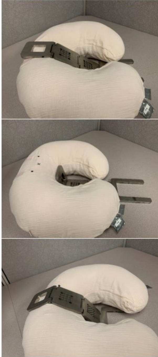
Figure 36. Example photos of the newborn device in a C-shaped nursing pillow in each position during lounging-intended use. Intended supine (Top), slouched (Middle), and prone / neck hyperextended (Bottom) positions.
