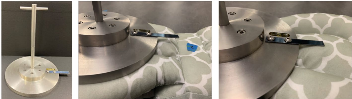
Figure 16. (Left) Firmometer device machined according to Australian/New Zealand Standard 8811.1:2013; (Center) Example of passed test with feeler arm not in contact with product; (Right) Example of failed test with feeler arm in contact with product.
