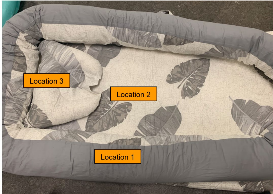
Figure 15. A sample of testing locations on a flat surface. Location 1 is at the maximum product thickness, Location 2 is at the minimum product thickness, and Location 3 is a subjective location of interest, which varies between products.
