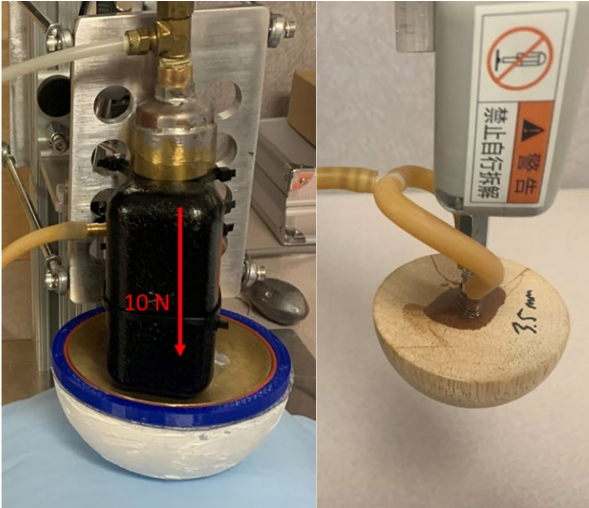
Figure 8. (Left) Attachment of 5 inch diameter hemisphere to original testing device with additional weight to achieve 10 N of thrust; (Right) Example of connection of airflow setup directly to Probe 6. The branch of the T-fitting connects to the digital barometer, and the run section of the T-fitting connects to the flowmeter.
