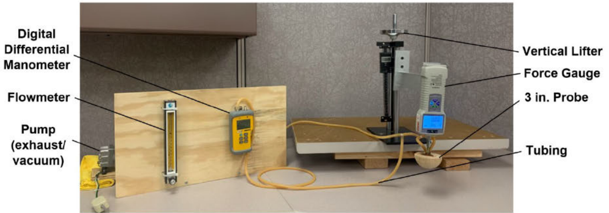
Figure 24. Airflow set up connected to the vertically guided lifter device.
